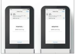
**8.** Results are displayed within 12 minutes of applying the sample. The left-hand image here shows a positive result for SARS-CoV-2 Ag and the right-hand image shows a negative result for SARS-CoV-2 Ag. Tap Finish to complete testing or tap Comment to leave a comment or to reject the Test, then follow prompts to return to the Home Screen. All test results must be read using the Lumiradx Instrument.
