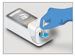
**6.** Apply **one whole drop** of the sample onto the **Test Strip Sample Application Area** when prompted by the **Instrument**.
